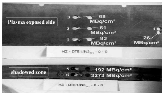
Fig. 1. Tritium content in different locations of the Mark-IIA JET divertor tile number 3 after the DTE1 campaign (including plasma exposed and plasma shadowed sides of the tile).
